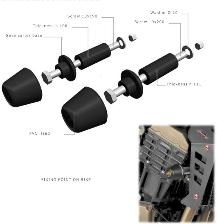
FIND THE FIXING POINT ON THE MOTORBIKE BEFORE START THE MOUNTING PROCEDURE. USE THE SPECIFIC THICKNESS AND BOLTS LIKE DESCRIBED INTO THE PICTURE TO OBTAIN THE RIGHT DISTANCE OF THE SAVE CARTER FROM THE MOTORBIKE. FIX THE PVC HEAD OF SAVE CARTER ONLY AFTER FIX AND LOCK ALL THE KIT.
