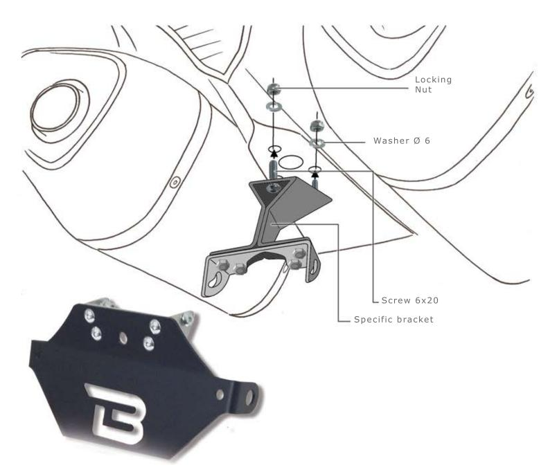
REMOVE THE ORIGINAL LICENCE PLATE AND APPLY THE BARRACUDA LICENCE PLATE IN THE SAME HOLES USING THE THREE ROUND HEAD 6X20 SCREWS OUTSIDE AND FIXING WITH THE NUTS INSIDE. WHEN YOU HAVE POSITINED THE SPECIFIC BRACKET YOU CAN APPROACH THE LICENCE PLATE.
